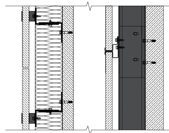
✓ Assembly system - mechanical, visible
